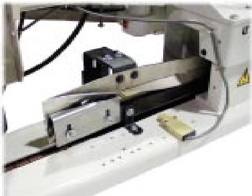
For all kinds of self-supporting bags, fold-over kit 93051FA folds the bag-top to the rear. It mounts easily on plain closure feed-in device GBR29905X1.
