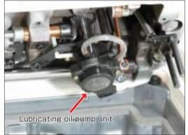
The top feed mechanism employs a grease tank and oil wick lubrication mechanism.
